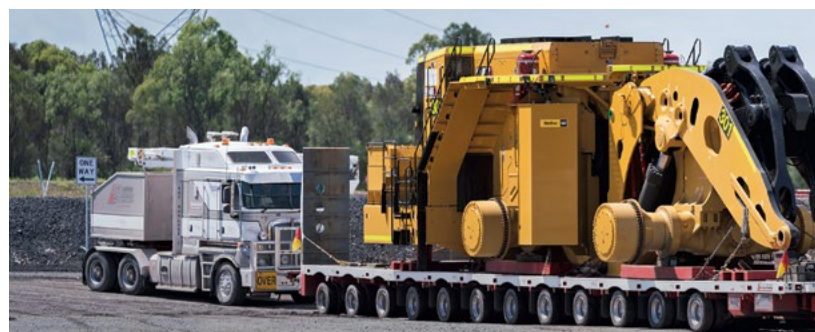
Prime mover trucks haul a road train to deliver a CAT 994K Wheel Loader to United Wambo JV, Hunter Valley, NSW
