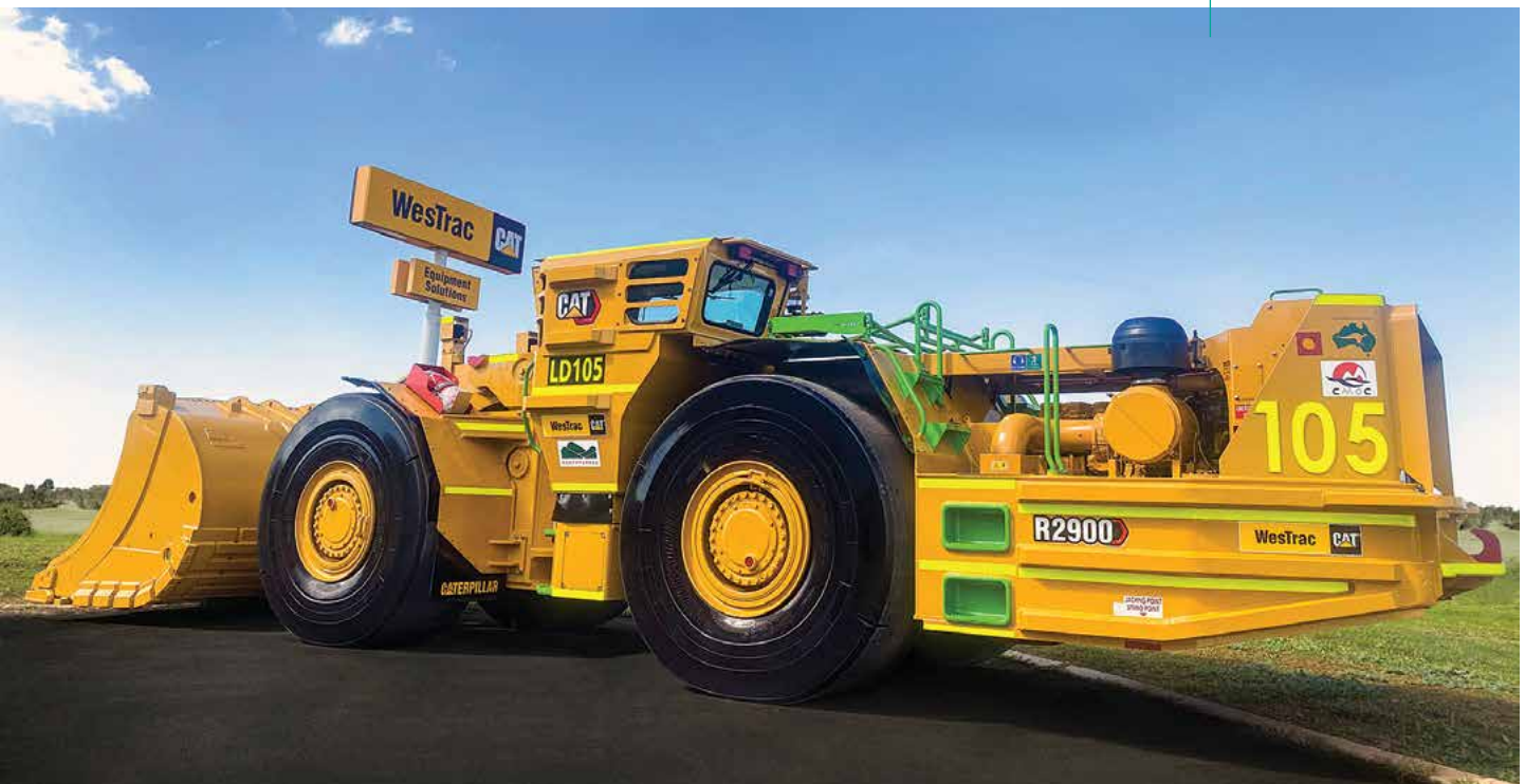
Northparkes Mines R2900G LD105 after a Certified Powertrain Rebuild by WesTrac Dubbo team.
