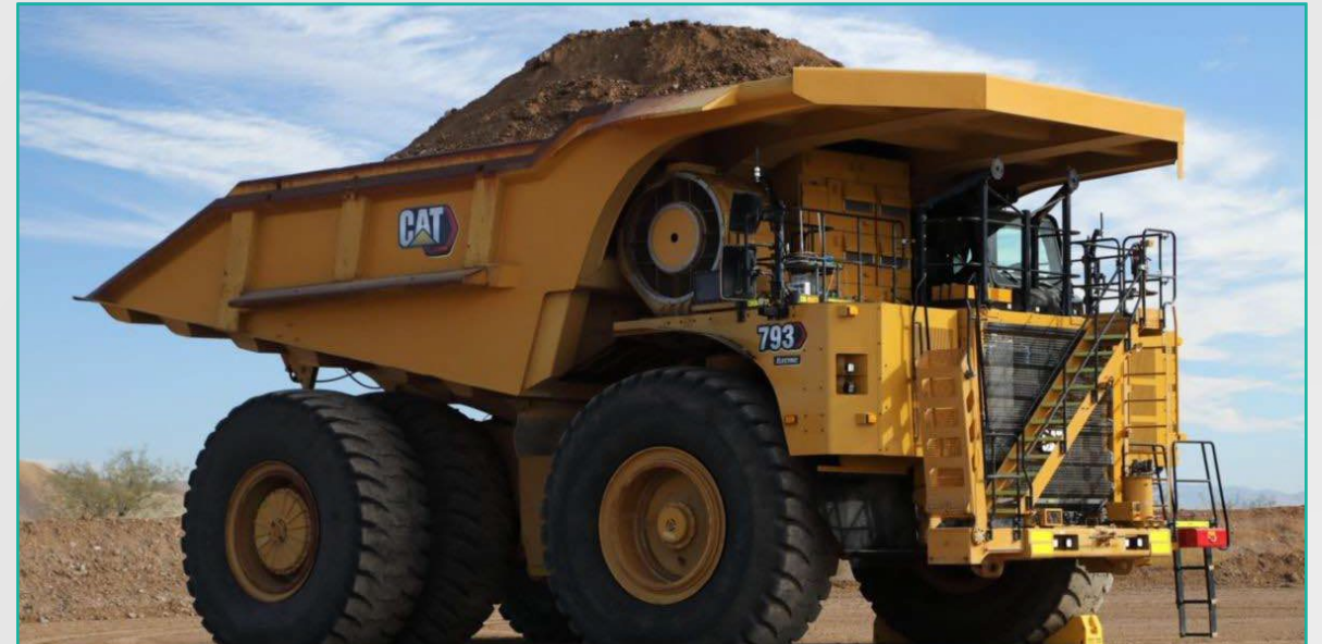
Caterpillar's first battery-electric 793 mining truck, Arizona Proving Ground, USA
