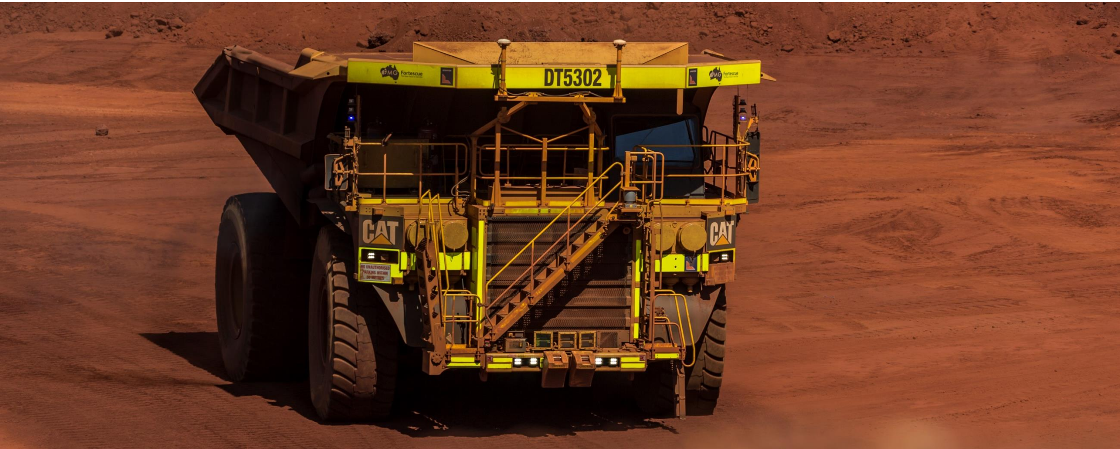
Autonomous 793F mining trucks have delivered productivity gains to FMG
